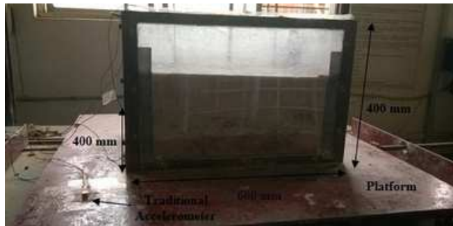
Fig. 1. Soil model container monolithically attached with shake table
