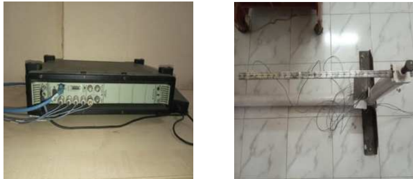
Fig. 1 (a) Bruel & Kjaer module, (b) Beam model
